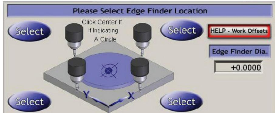
Fig 35: Probe settings on the Offsets screen.
