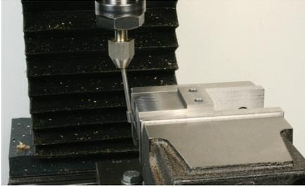
Photo 66: A conventional wiggler detects the position of the face of the workpiece.
