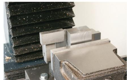
Photo 61: Using a square to set an edge vertical by referencing off the top of a vice jaw.
