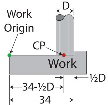
Fig 36: Calculating the position of the CP when creating the step.
