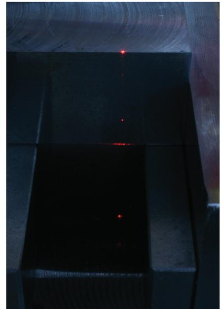
Photo 69: Splitting the dot on the edge sheds light down the edge and onto the vice base.
