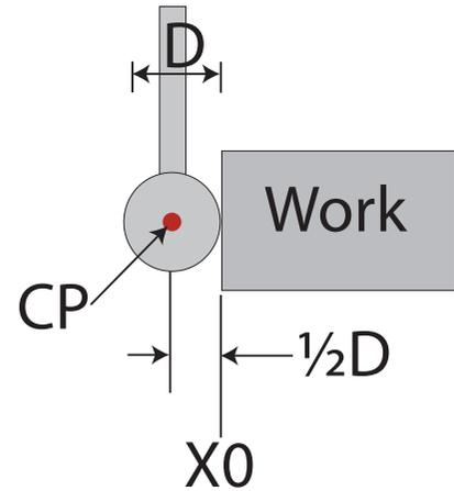
Fig 34: A touch point sensor indicates when the CP is half the diameter away from the workpiece.
