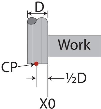
Fig 32: Position of the CP along the X axis as the cutter touches the paper.
