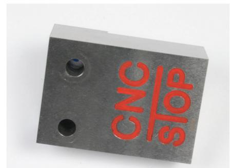
Photo 72: Lettering cut in the side of the stop.
