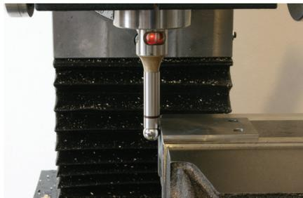
Photo 65: A probe lights when it touches the work.
