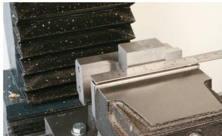
Photo 62: Using a ruler to position the work.
