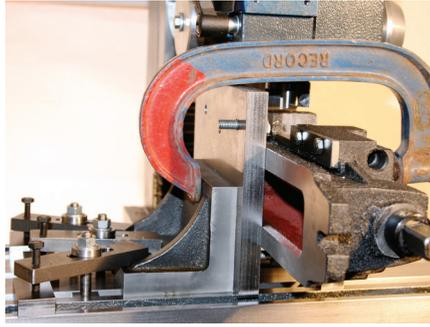
Photo 70: Support the vice on its side against an angle plate.
