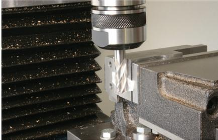
Photo 64: A cutter is half its diameter away from the work when it touches the paper.
