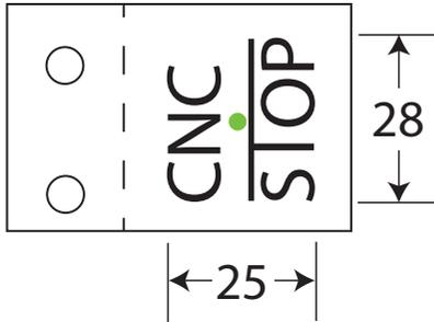
Fig 38: The position of the lettering.
