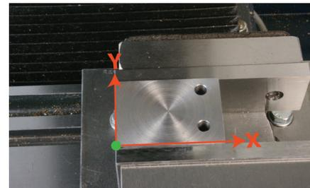
Photo 63: The green dot shows the work origin at the front left corner of the top face of the workpiece.
