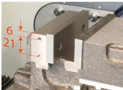
Fig 37: The hole positions.
