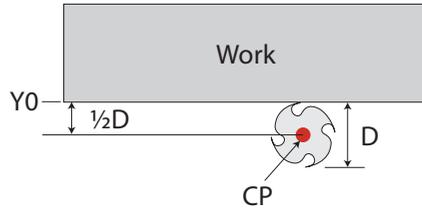
Fig 33: Position of the CP along the Y axis as the cutter touches the paper.
