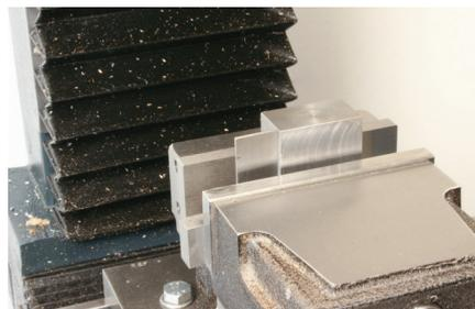
Photo 60: Using a square to set an edge vertical by referencing off the inside bottom surface of the vice.
