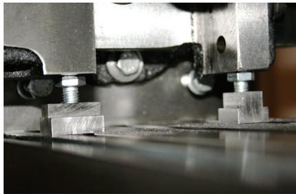
Photo 71: Support the vice casting using jacks.
