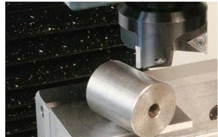
Photo 58: Using a roller of known diameter for height setting.
