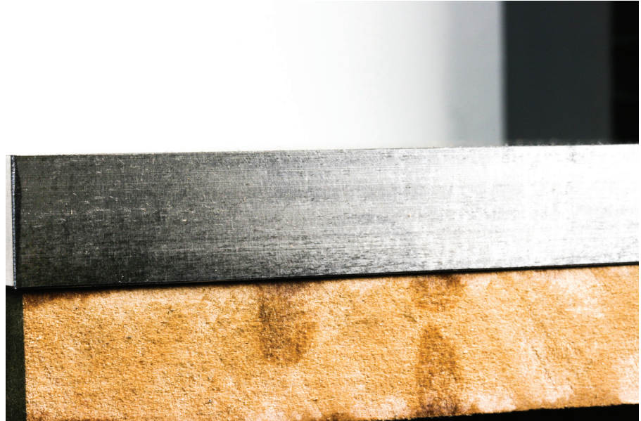
Photo 44: surface finish from the side of an end mill..
