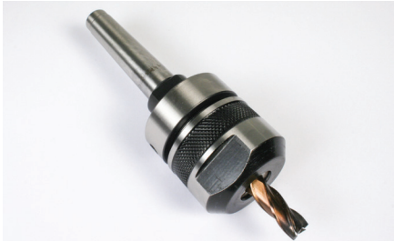
Photo 38: Pozilock collet chuck..
