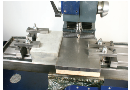
Photo 34: Butting a plate against a flat faced block previously set parallel to the Y axis..
