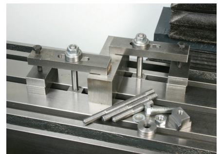
Photo 36: Clamps studs and T-nuts..
