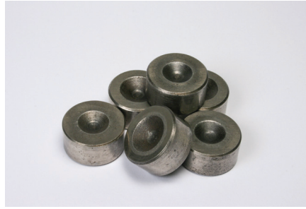
Photo 32: Engine tappet pads for use as spacers.
