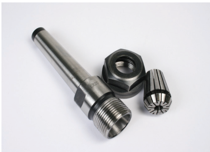
Photo 41: Component parts of the ER collet chuck.
