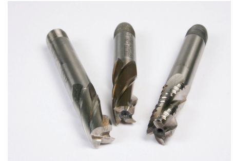
Photo 42: Roughing and finishing end mills..
