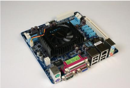
Photo21: A modern single-board computer with a parallel port..
