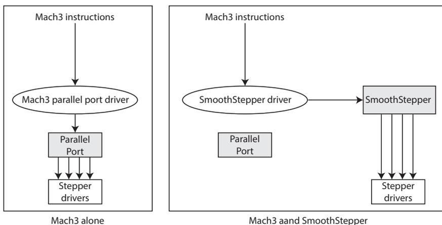
Fig 8: Signal path diverted by SmoothStepper driver.
