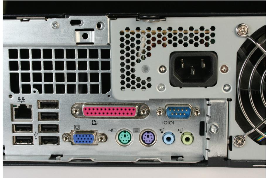
Photo 20: The large, pink, 20 way parallel port (printer) connector.
