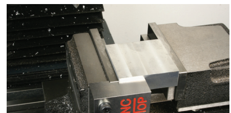
Photo 76: Block located against two fixed edges.
