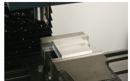
Photo 74: The block sitting on parallels and gripped in the vice..
