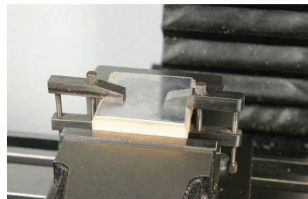
Photo 75: Sheet on a backing, ready to have the corner holes drilled.
