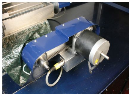
Photo 9: Stepper motor on the Y axis.
